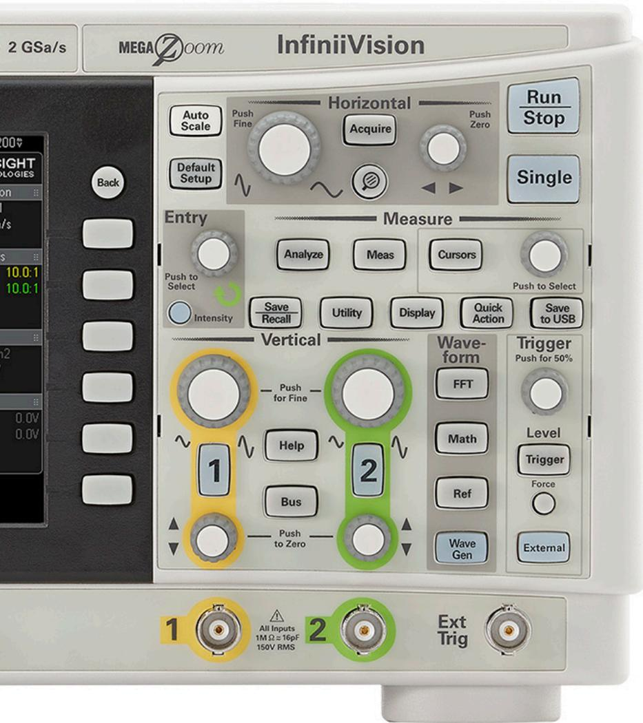
Custom measurements are easy with “Cursors.” Measure any value or the difference using four powerful cursors.
