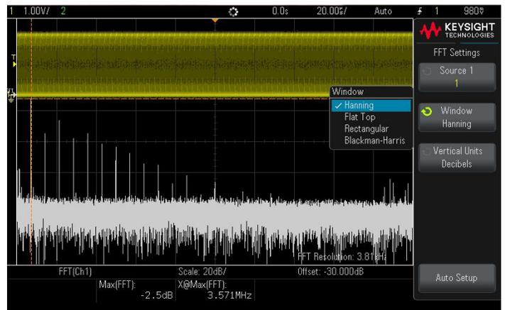
Multiple FFT window functions are supported to provide required signal analysis.
