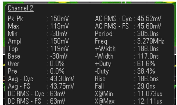
Snapshot of all 24 measurements being taken simultaneously.
